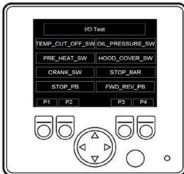
P2 shows I/O tests. Tests all functions and safety controls.
