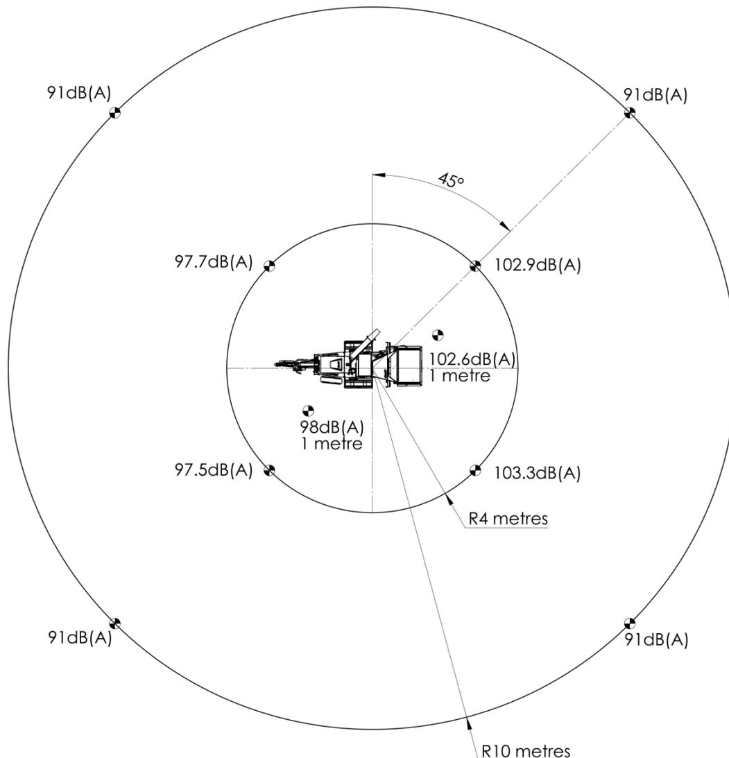
A-weighted emission sound pressure (beside operator's ear)  $L_{pA} = 111.7\text{dB(A)}$ .
