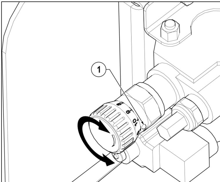
1 CONTROL VALVE FEED SPEED ADJUSTMENT. POSITION INDICATED BY PIP. 0 = MINIMUM 10 = MAXIMUM
