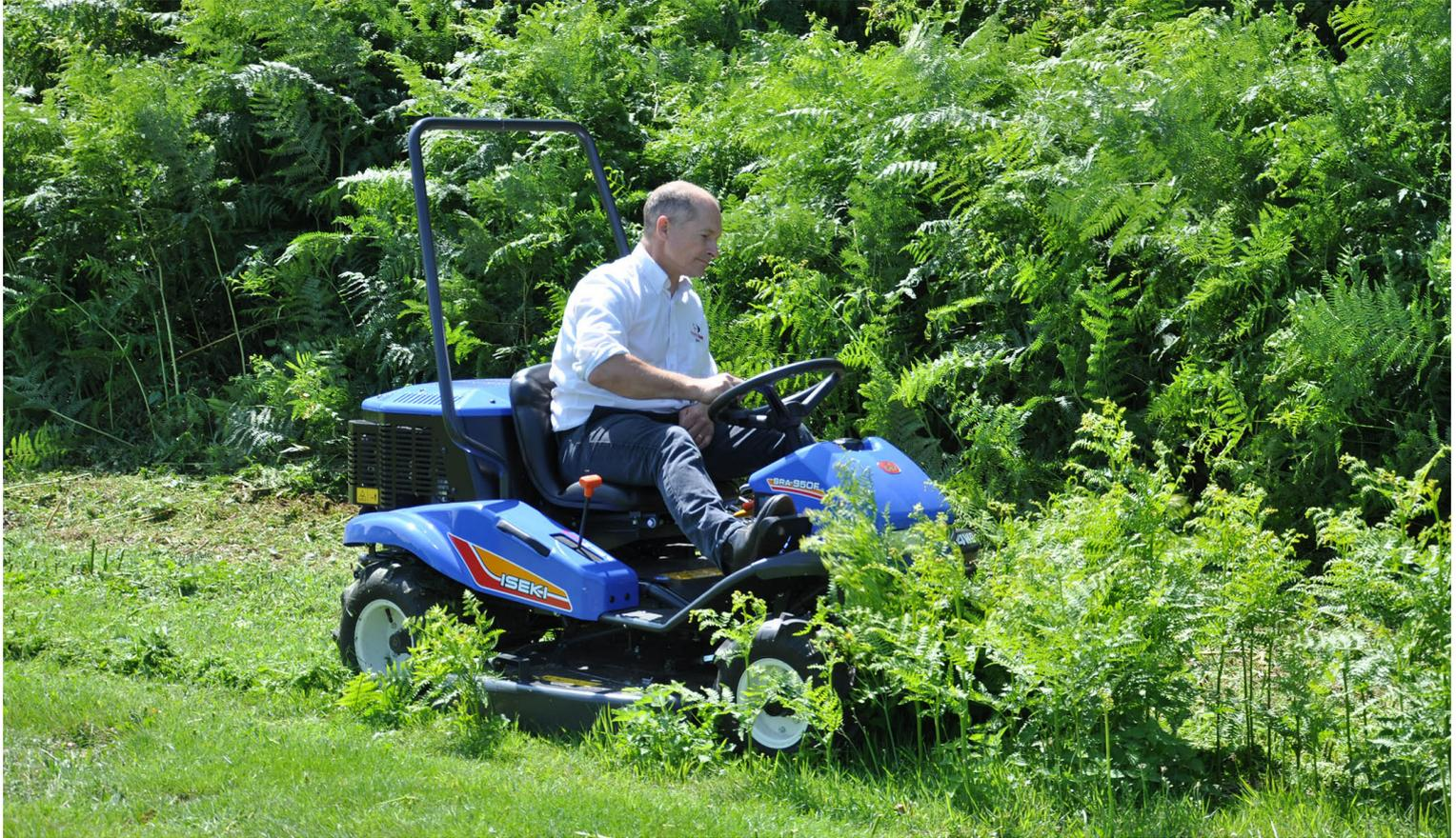
The SRA800 and SRA950F are ride-on brush cutters capable of cutting grass and thick vegetation right up to saplings. Their low height aids stability when used on slopes.
