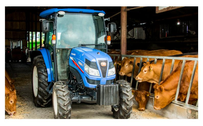
The TG6495 and TG6375 feature the new IQ Dual-Clutch transmission that offers the control of a manual with the convinience of an automatic. There are 8 main gears and 3 ranges. Gears are changed by simply moving the gear lever through the straight shift gate. If 'D' is selected then gears 4-8 are operated automatically - ideal for roadwork or towing.
