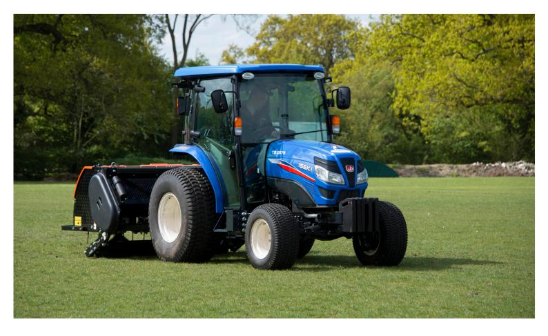
The TG6675 PS compact tractor is available with a ROPS or a factory fitted, fully air-conditioned category 2 cabin. It features a 65hp four cylinder, Stage IIIB diesel engine, with a F12/R12 power-shuttle transmission. The rear, category 1 & 2, 3-point linkage has a capacity of 1,600kg at ball end and 1,500kg at 24 inches.
