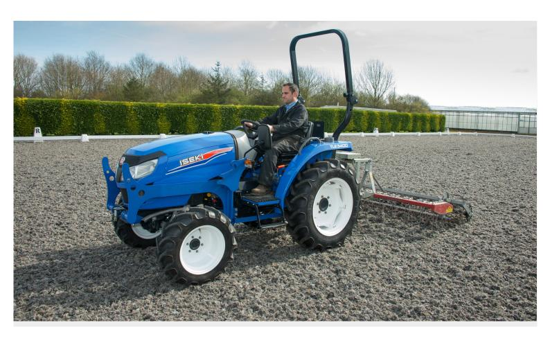
The TLE3400 is ISEKI's premium economy tractor. The 38hp tractor has a three speed hydrostatic transmission and a lift capacity of 1000kg. It is supplied with agricultural tyres or turf tyres as standard.
