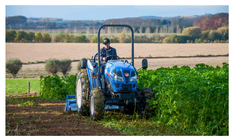
The ISEKI TLE4490, the latest addition to the Premium Economy range, features a 46hp 4 cylinder diesel engine, F8/R8 synchro shuttle transmission, rear PTO 540rpm, an auxillary valve, three point linkage with 1,200kg capacity at the ball end and 1,100kg at 24 inches.
