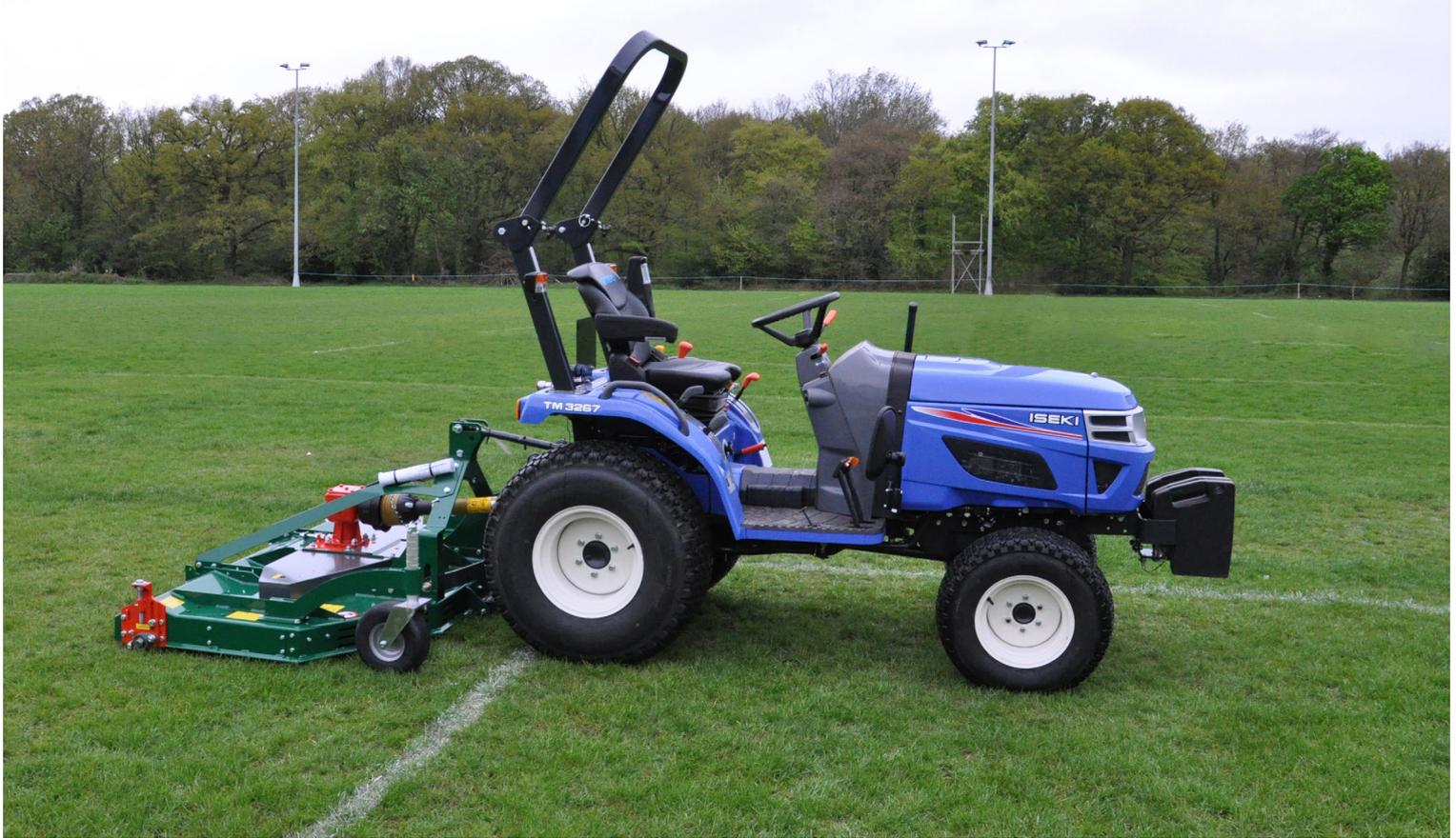
The new ISEKI TM3267 is a versatile 25hp diesel compact tractor with a F8/R8 mechanical transmission. The ISO-mounted operator's platform combined with ergonomically positioned controls ensures operator comfort during extended working periods. The 3-point linkage has a lift capacity of 600kg or 800kg (TM3267 only) when fitted with the high-capacity lift kit.
