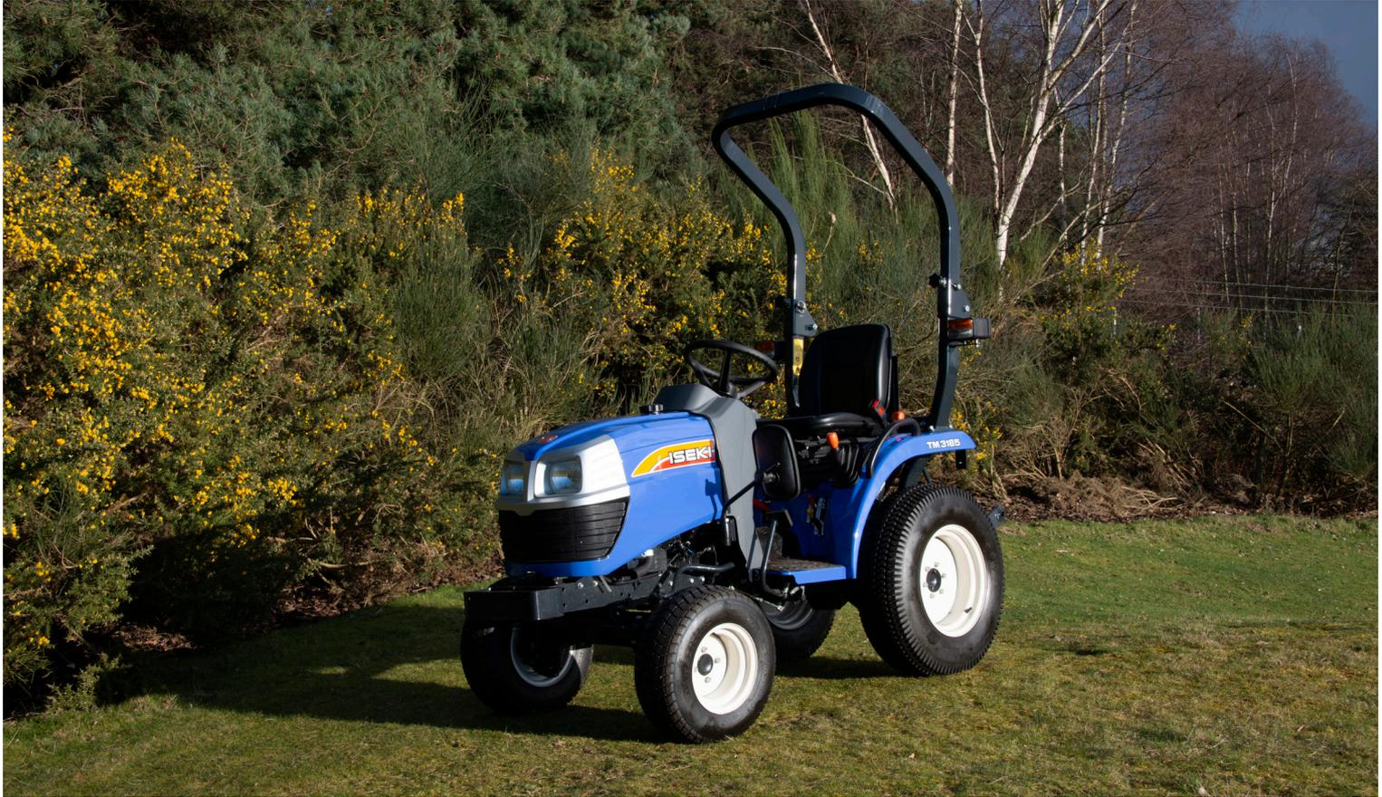
The ISEKI range of compact tractors are great all-round machines for both private and professional users. The TM3185 is ISEKI's most compact tractor with a 16hp engine, four wheel drive, power steering and compact dimensions, making it the ideal workhorse for restricted environments.
