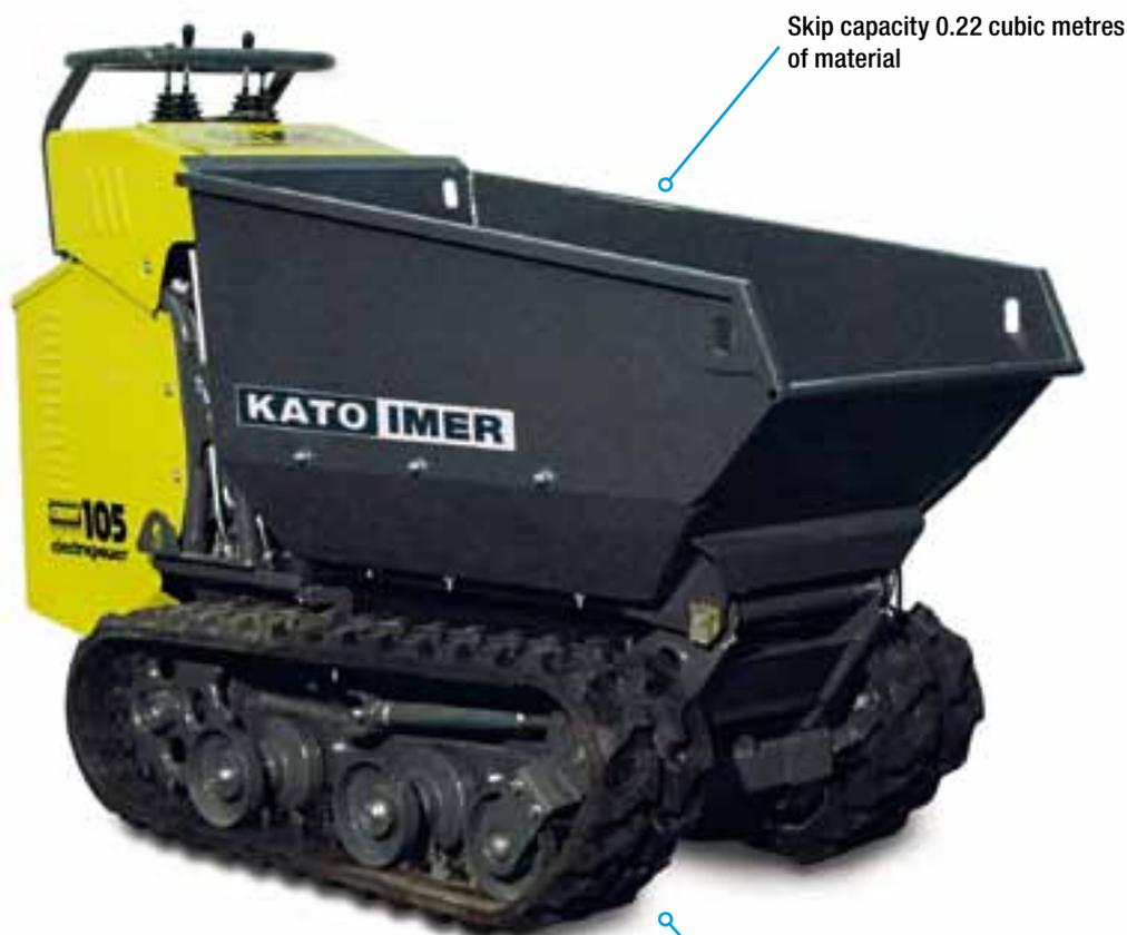
Skip capacity 0.22 cubic metres of material
