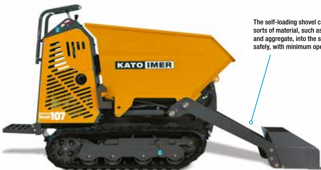
The self-loading shovel can transfer all sorts of material, such as rubble, earth, and aggregate, into the skip quickly and safely, with minimum operator effort
