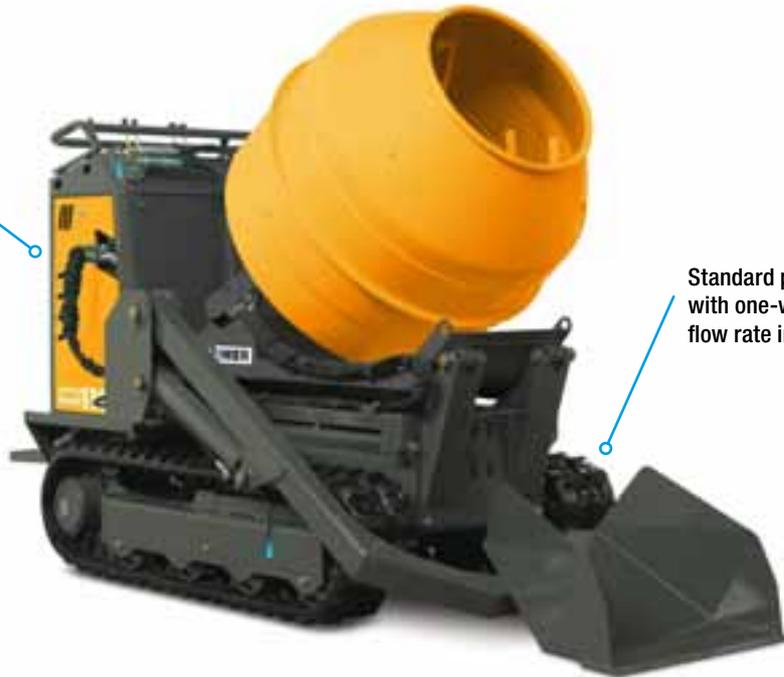
Standard power take-off with one-way or two-way motion and flow rate increased to 26 L / min
