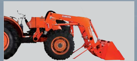
2 Boom Fulcrum Upper: Height position Bottom: Power position
