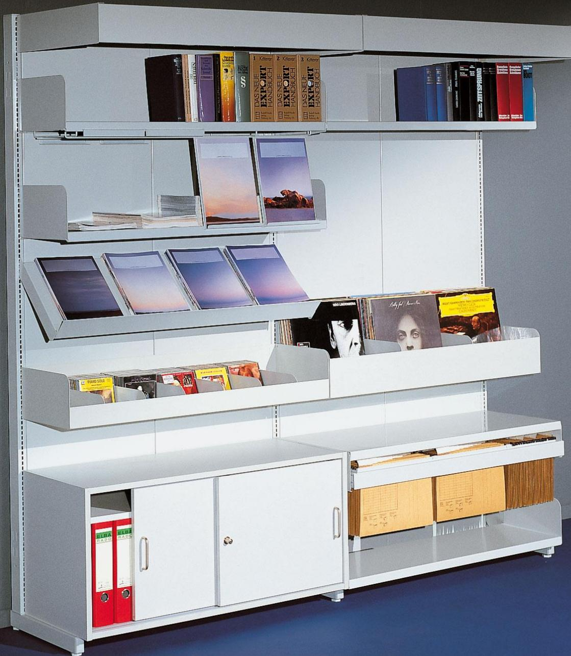
Universal screwless shelving without any front uprights to allow easy access to books. Takes minutes to assemble. The steels can be adjusted in 16mm increments. Each bay can have shelves of different depths or construction. Premium steel in a powder coated Light Grey finish. Shelves have a weight loading of 80 – 100kgs depending on depth
