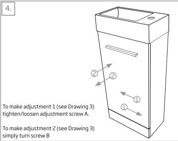
Hinges may require adjustment for correct door alignment. This is achieved with the adjustable soft close hinges using the adjustment screws A and B (see Drawing 3).
