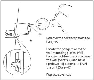
Fascias may require adjustment for correct alignment. This is achieved with the adjusting mechanisms shown below.
