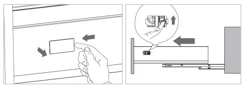
Remove fascia - turn release mechanism on both sides after removing cams under drawer
