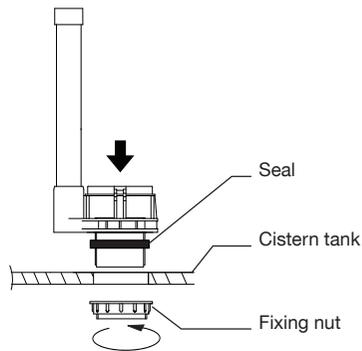
Insert flush valve body into flush valve seat, turn it clockwise until you hear a "click"
