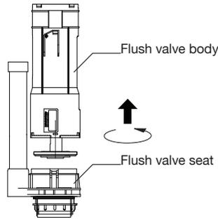
Install flush valve seat and seal as shown
