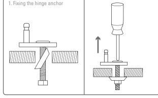
Assemble the components as shown, and push the butterfly fixing, fixing nut and fixing screw through the seat fixing holes in the pan. Pull up slightly on the base of the hinge anchor to engage the butterfly clip on the underside of the pan and tighten with a screwdriver to secure the hinge anchor into place.
