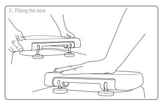
Align and insert the hinge anchors into the hinges on the seat and firmly press down until you hear them click into position. Adjust the hinge anchors to make sure the seat lines up with the edges of the toilet pan. When you are satisfied the seat is in the correct position, remove the seat from the hinge anchors (see step 3) and fully tighten the screw in the top fix insert (shown in step 1). Place the cover plates over the hinge anchors. Replace the seat and 'click' into position.
