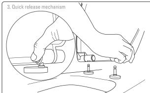
This toilet seat is designed for quick and easy removal when cleaning the toilet pan. To activate the quick release lift the lid and seat up. Press the buttons one by one and lift the seat up. To replace the seat align the sockets with the pins and firmly press down until you hear them click into position.
