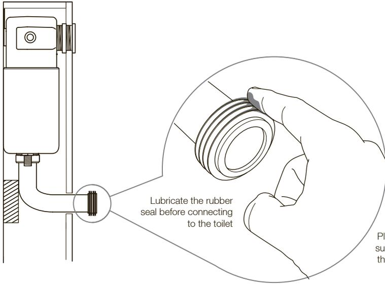
Lubricate the rubber seal before connecting to the toilet
