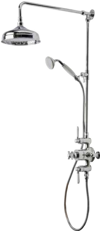
Regatta exposed dual function shower valve with shower head and handset TR3015 • Thermostatic sequential shower valve • Separate flow control to shower head and handset • Brass adjustable length rigid riser rail and shower arm • 200mm brass shower head • Minimum recomended pressure 0.5bar • 10 year guarantee includes thermostatic cartridge £560.00
