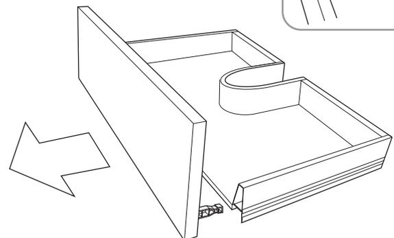
NOTE - When replacing the drawers back on their runners ensure they have been 'clicked' back into position at point A in diagram 6 (on both sides)
