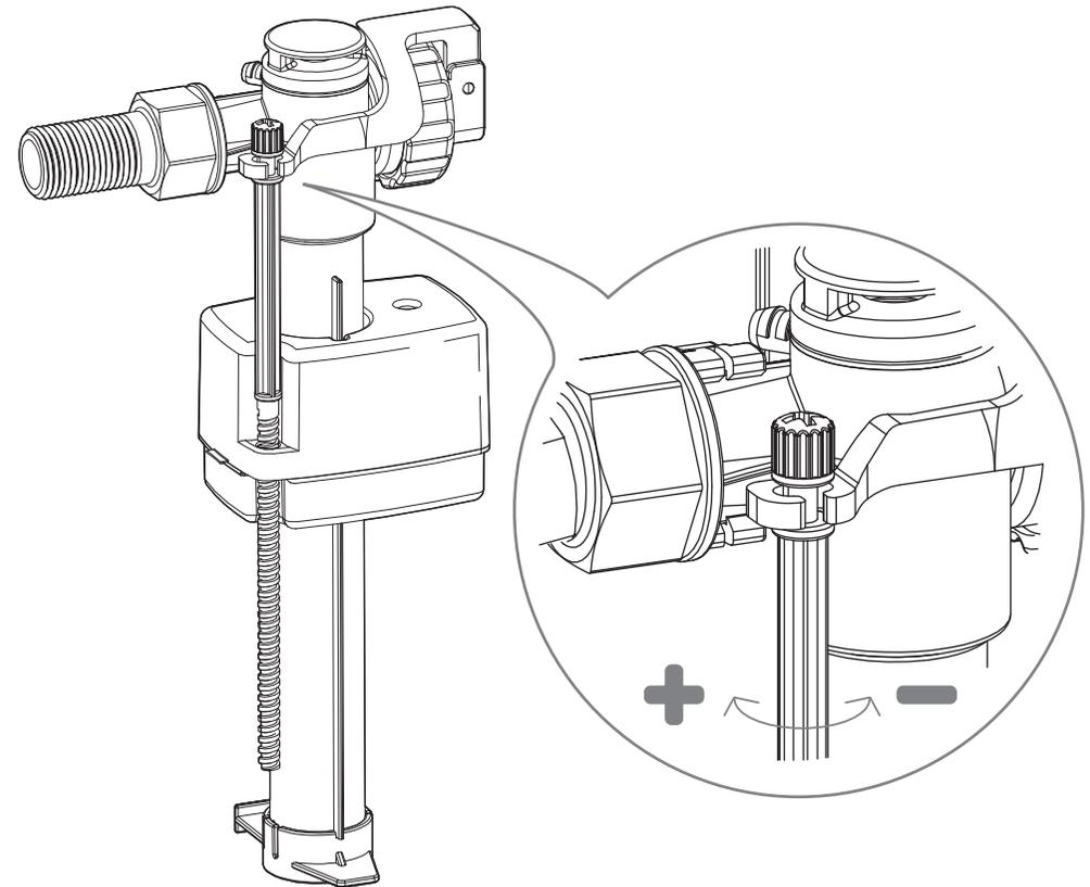
By adjusting the fill valve the water level can either be increased or decreased accordingly
