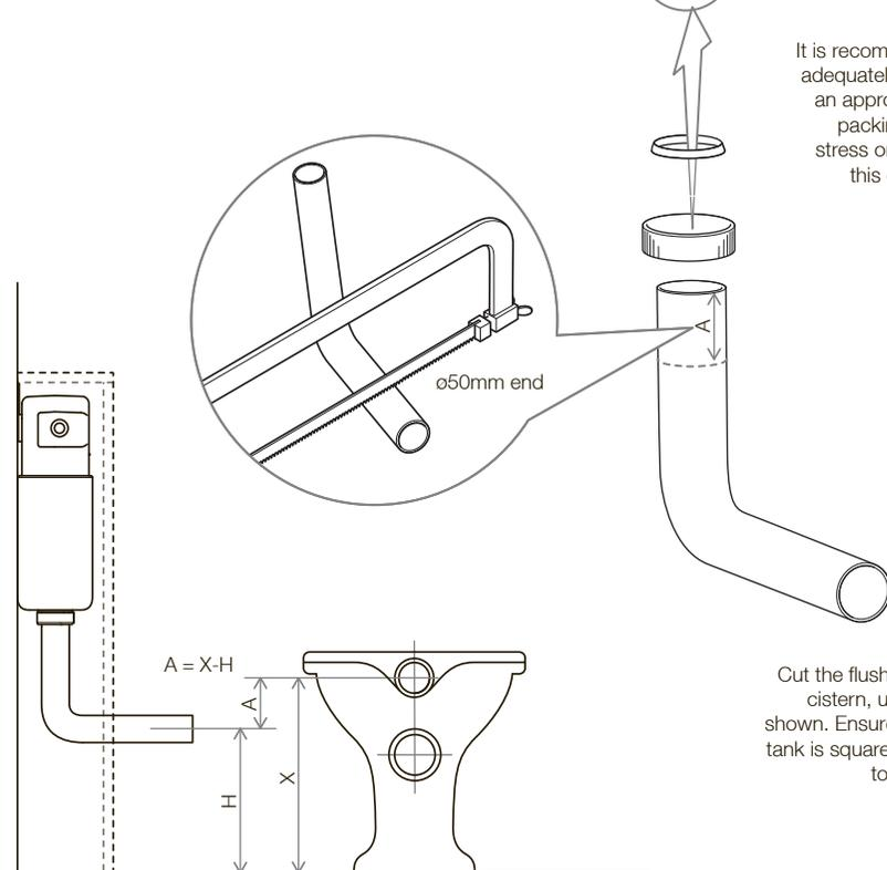
Cut the flush bend to size and attach to the cistern, using the appropriate fittings, as shown. Ensure alignment to pan from cistern tank is square both vertically and horizontally to allow seal to function correctly
