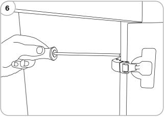
If the delivered configuration isn't suitable, remove door and hinge plates from unit using a suitable tool.
