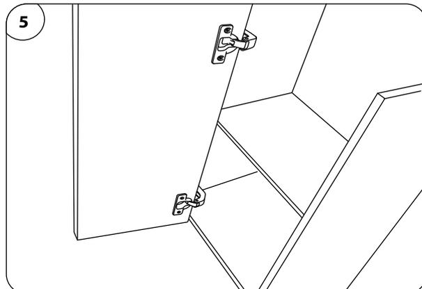
Reattach the door to the chosen side and replace cover caps in the obsolete hinge holes.
