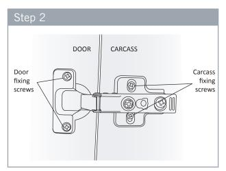
Choose the desired handing and fix hinges to the door and then the carcass. Holes are also provided on both ends of the door for the badge attachment to be fitted once the desired hinge position is chosen.
