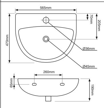
DIAGRAMS NOT TO SCALE | ALL DIMENSIONS IN MM | TOLERANCE OF  $\pm$  5MM SLOTED FIXING HOLES (30MM X 20MM APPROX)
