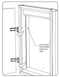
R1) In order to secure the cabinet in a recess, a 10mm hole has been pre-drilled on each of the inside faces of the cabinet to accept screws that will secure into the framework (use screws that are suitable for the framework). These fixing points are concealed behind the upper hinge locations so the hinges and door(s) will need to be removed before installation. Unscrew the hinge and door assembly and keep the screws in a safe place. It may also be useful to remove the shelf brackets.
