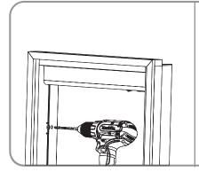
IF ACCESS IS POSSIBLE DRILL THROUGH THE PILOT HOLES FROM THE INTERIOR OF THE CABINET TAKING CARE TO STAY PERPENDICULAR TO THE CABINET SIDES. THE DRILLED HOLE SHOULD BE CONCENTRIC TO THE PILOT HOLE. AVOID DRILLING THE HOLE ON AN ANGLE. DRILL A HOLE LARGE ENOUGH FOR THE SHANK OF THE SCREW BEING USED, BUT NOT LARGE ENOUGH FOR THE SCREW HEAD TO FIT THROUGH.
