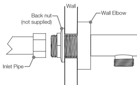
1. Secure wall elbow in place using the back nut provided (See diagram)
