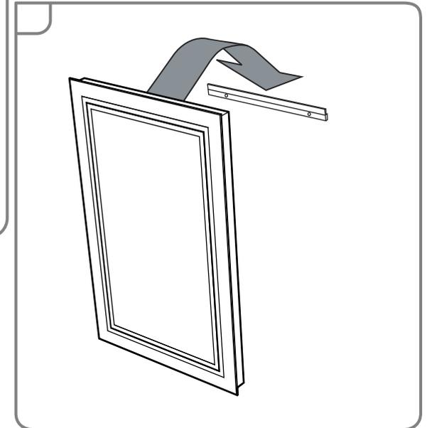
Mount the Mirror onto the fixing bracket fitted to the wall. The fixing bracket will inside the frame of the mirror. This mirror can be installed in a portrait or landscape orientation. To ensure the mirror is securely mounted, add a bead of silicone to the bottom edge where the mirror meets the wall.
