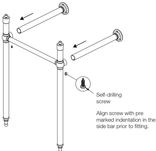
**2** Centrally align the washstand and adjust the extension appropriately.
