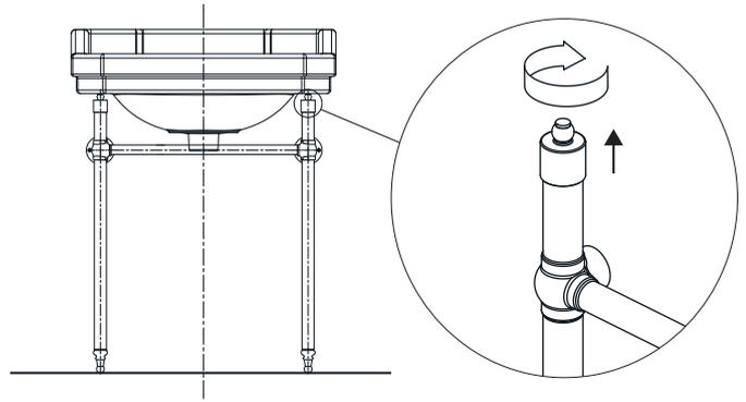
**3** Once the washstand is aligned and level, mark out and drill the pilot holes. Insert the wall plugs and using the screws provided attach the washstand to the wall.
