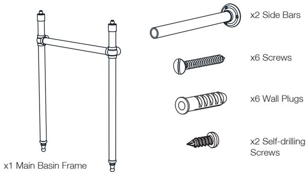
**1** Attach the side bars using the self-drilling screws provided.
