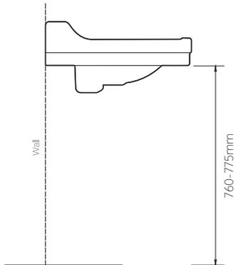
Ensure the basin is firmly screwed to the wall using appropriate basin fixings before proceeding. Fix the basin in accordance with the fixing manufacturer's instructions.
