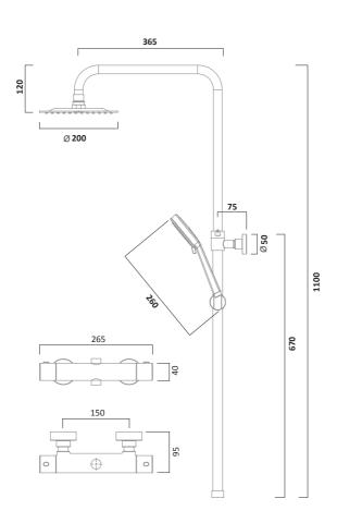
Cool Touch Thermostatic Dual Function Bar Valve with Shower Head & Handset
