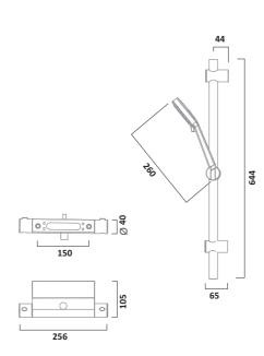
Thermostatic Single Function Bar Valve & Handset Chrome SQT1916
