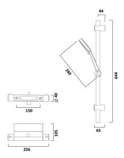
Thermostatic Single Function Bar Valve & Handset Chrome SQT1916
