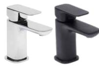
Haze Basin Mixer with Click Waste Minimum recommended pressure 0.2bar 52(w) × 132(h) × 133(d)mm
