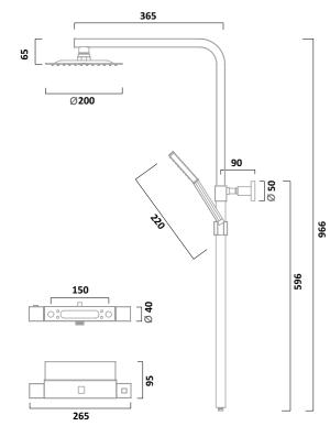
Thermostatic Dual Function Bar Valve and Accessory Shelf with Shower Head & Handset Chrome SND2008
