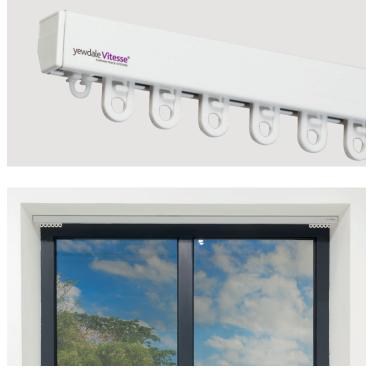
The roller runners are the real star of the show, situated as 12 per linear metre and providing a secure hold on the curtain. The roller runners themselves are a supremely capable component, with two smooth running wheels located either side of the plastic eyelet. The wheels sit either side of the gap in the track, locked in. As a result, this track holds up well with heavy use and is robust enough to withstand the rigours of day to day use.
